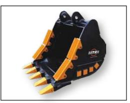
For extreme applications, we also manufacture Heavy Duty and Rock buckets. HARDOX super high strength wearable steel, with ITR teeth and adapters maximize product's reliability, excavation performance and economical efficiency. These greatly reduce the time and cost of maintenance thus improving working efficiency.
