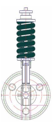
ITR RANGE OF RECOIL SPRINGS FOR EXCAVATORS AND DOZERS
