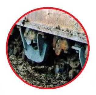
ITR recommends track guards only when the excavator is being used in rocky working conditions (not in normal working conditions) as they are specifically designed for this.
